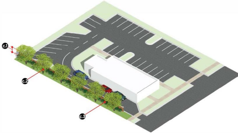
Figure 13-1-132(6): Drive Through Screening
